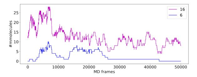
The above plot shows number of water molecules (or paths) in cluster 16 and 6 throughout the simulation. One can observe that number of molecules in cluster 6 diminishes approximately in the middle. This kind of plot can be easily generated with additional CSV data.
