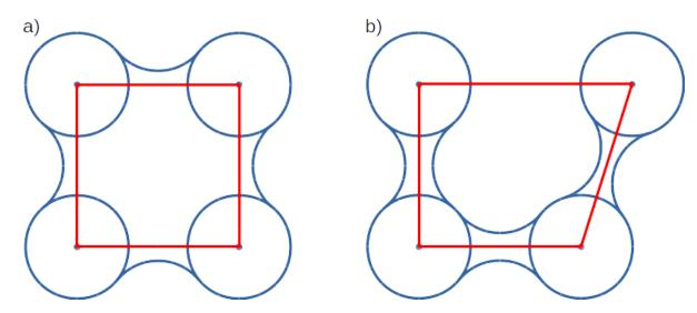
Convex hull (red shape) of atoms (blue dots with VdW spheres) and SES (blue line): a) convex hull and SES cover roughly the same area, convex hull approximates SES; b) movement of one atom dramatically changes SES, however, interior of the molecule as approximated by convex hull remains stable.
